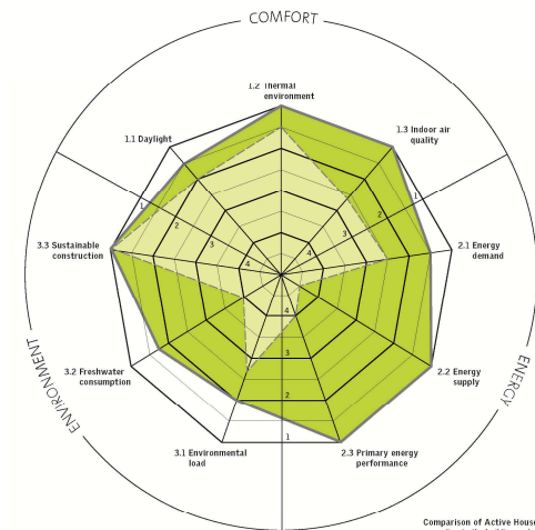
Comparison of Active House and standard house built according to the building code. ■ Calculated performance of the Great Gulf Active House ■ Standard house built according to the building code.
